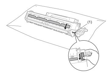
Wipe the surface of the drum gently with a dry cotton swab until the dust or glue on the surface comes off.
