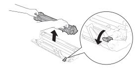
8 Place the toner cartridge back into the drum unit until the lock lever lifts automatically.
